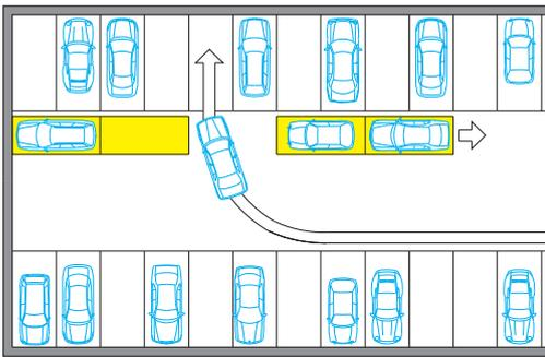
Occupied parking platforms are shifted by means of hold to run device until parking places behind or in front of/opposit of them can be crossed.
