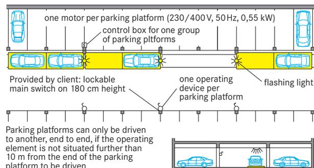
The electrical components supplied by the manufacturer must be connected in accordance with the appropriate wiring diagram and local regulations. German VDE electrical requirements must be adhered to, in order to validate the TÜV tested circuit.
