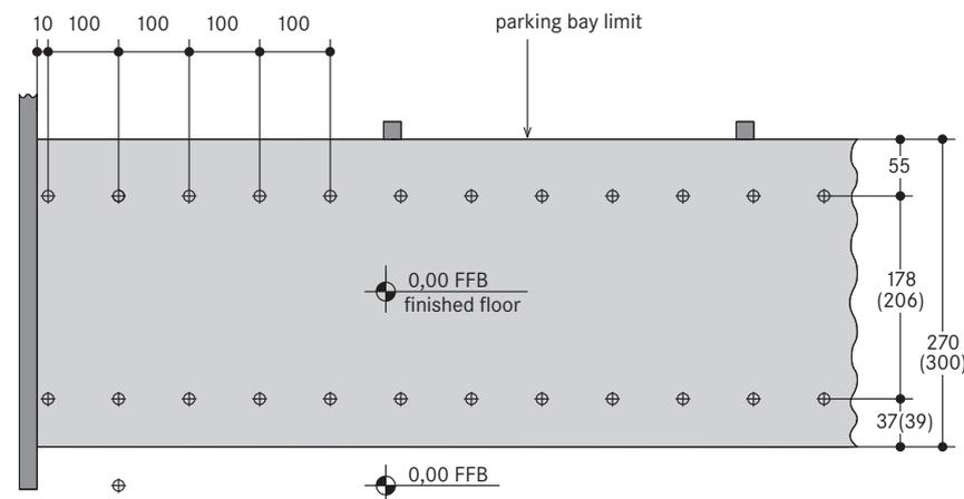
⊕ Measuring points at 100 cm points for checking unevenness acc. to DIN 18202, table 3, line 3, or acc. diagram
