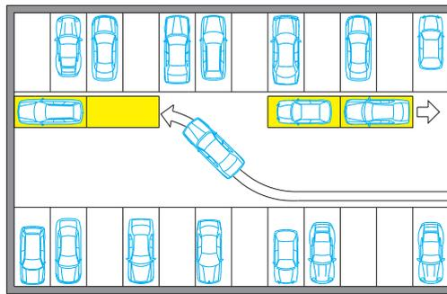
Parking places on platforms are directly driven onto or the parking platforms are shifted so that enough driving space is available to drive onto and park.
