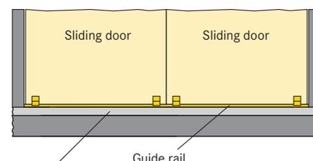
Finished floor level compliant to DIN 18353, floor evenness compliant to DIN 18202 table 3, line 3.
